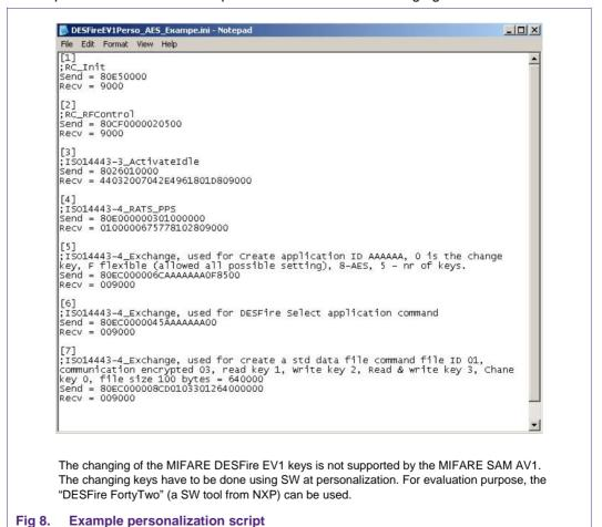
The keys of the application are by default 16-byte 00s and crypto option is AES as set in step 5 of the script file. Figure 9 shows the TestWinScard GUI after running the script.
