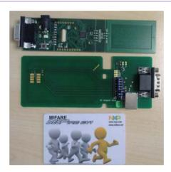
Fig 1. From top to bottom: Evaluation board [H\_EVB6], Smartcard contact adapter [H\_CASC] and Mifare DESFIRE EV1 card
